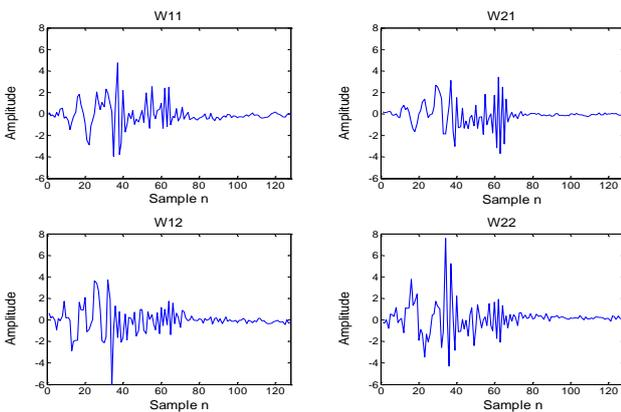
Fig. 7. Inverse filters are calculated by the Kalman filtering algorithm. (a)  $W_{11}$ ; (b)  $W_{21}$ ; (c)  $W_{12}$ ; (d)  $W_{22}$ .
