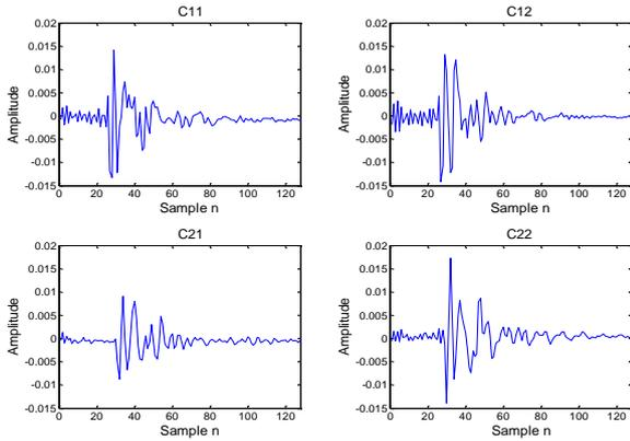
Fig. 6. Measured impulse responses in a vehicle cabin.
