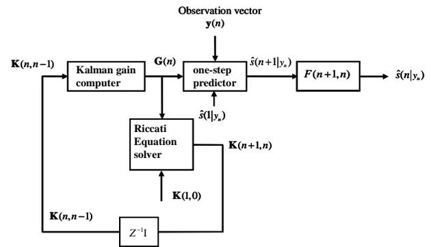
Fig. 4. Block diagram of the Kalman filter based on one-step prediction.
