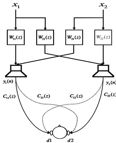
Fig. 1. Crosstalk cancellation system using the inverse filtering method.
