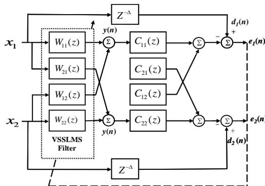
Fig. 2. Structure of crosstalk cancellation system using the VSS LMS error algorithm.
